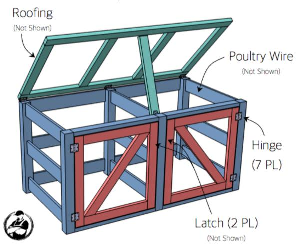
Attach roofing to **lid** using **1" roofing screws**.
